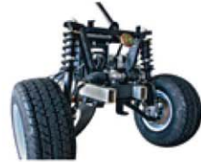
INDEPENDENT SPRING FRONT SUSPENSION
